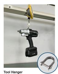
The tool can be attached EYFA41B to the balancer in the appropriate
